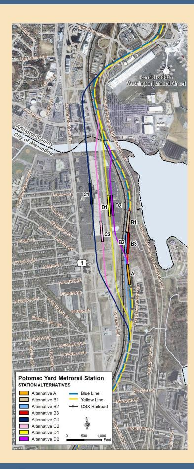
alignments west of the existing parallel CSX freight rail tracks. All of the station alternatives included in the previous study have been identified for consideration in the EIS scoping process. Additional alternatives may emerge as a result of the scoping process.
